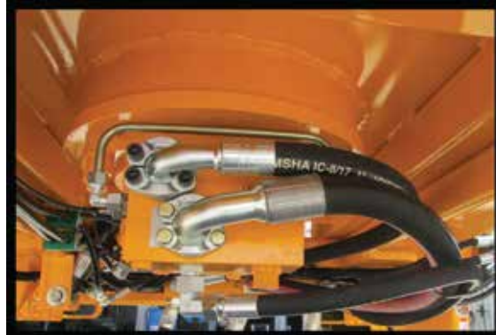
Heavy Duty Hydraulic Motor Drive for M2200 Pan Mixer
